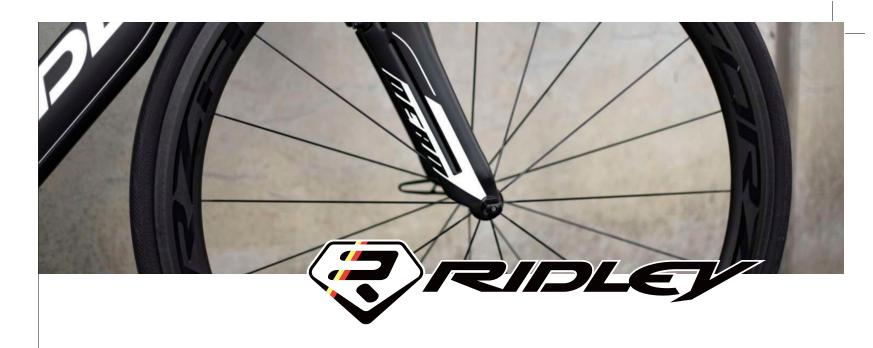
Our innovative F-Split Fork counteracts wind turbulence generated by the turning wheels. It does this by expertly guiding airflow through the split, down the fork arms, and away from the spokes. Decreased air
